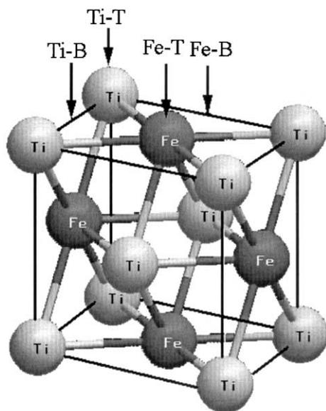
Fig. 6. The calculated H adsorption sites on the TiFe (110) surface. Ti-T and Fe-T denote H adsorbed on-top of Ti or of Fe atoms and Ti-B and Fe-B mark H adsorbed on a bridged site between Ti or Fe atoms.
